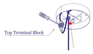
Thred the parts as shown and close the terminal block. Cable tensioner **Stainless Steel Cable** Ceiling rose cover Cable lock DISC 60CM Cable tensioner Pluggable Terminal Block
