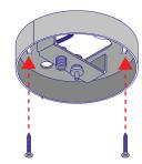
Run the electrical wire via the nipple that fixed at the ceiling rose.
