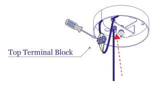
Thred the parts as shown and close the terminal block. Cable tensioner **Stainless Steel Cable** Ceiling rose cover Cable lock Top shade cover Cable tensioner Pluggable Terminal Block
