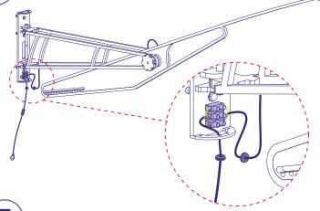
Fix the other side of the hanger covers by using supplied bolt as shown. Push the silicone button in to it's designed holes.
