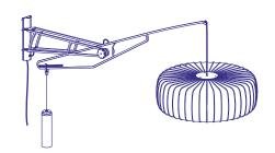
Thread the elect. core through the silicon button and connect it to terminal block as shown
