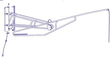
Fix one side of the hanger covers by using supplied bolt as shown.
