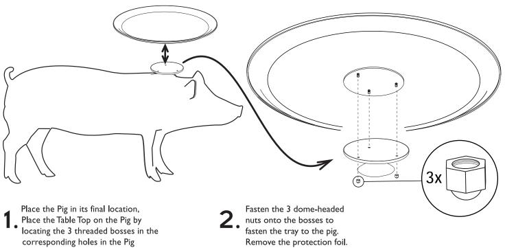
Note: Due to limited accesibility, Moooi suggests first tightening the nuts with fingers and then with a 10mm ring spanner or similar.
